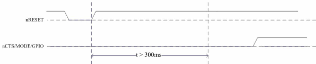
figure4-2 Normal startup mode
