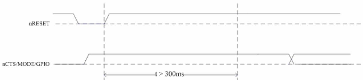
figure4-3 launching configuration mode
