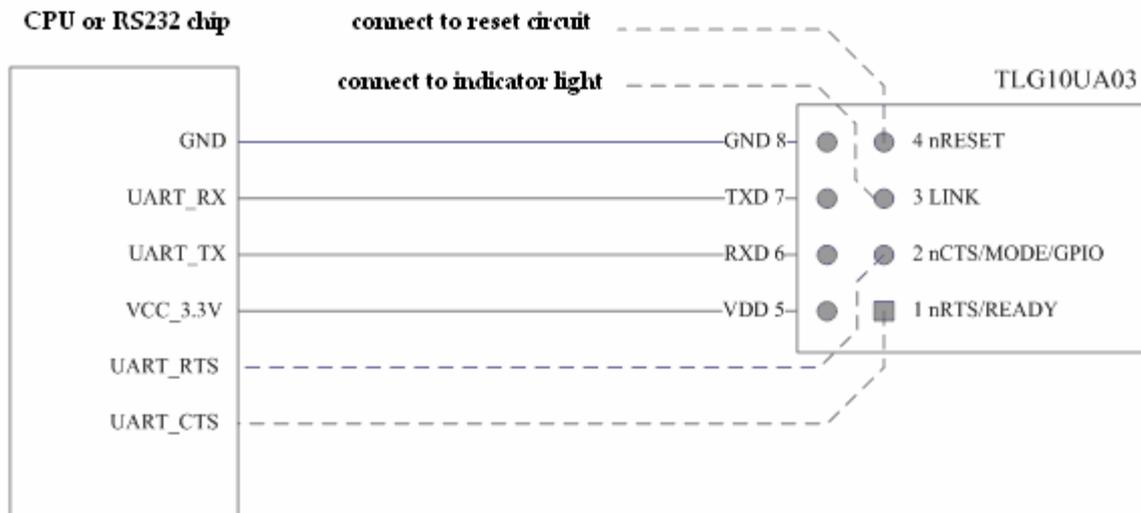
figure4-1 Hardware Connection
