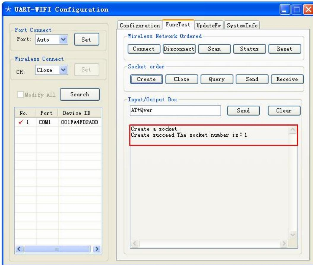
figure5-13 interface of the result of creating socket
