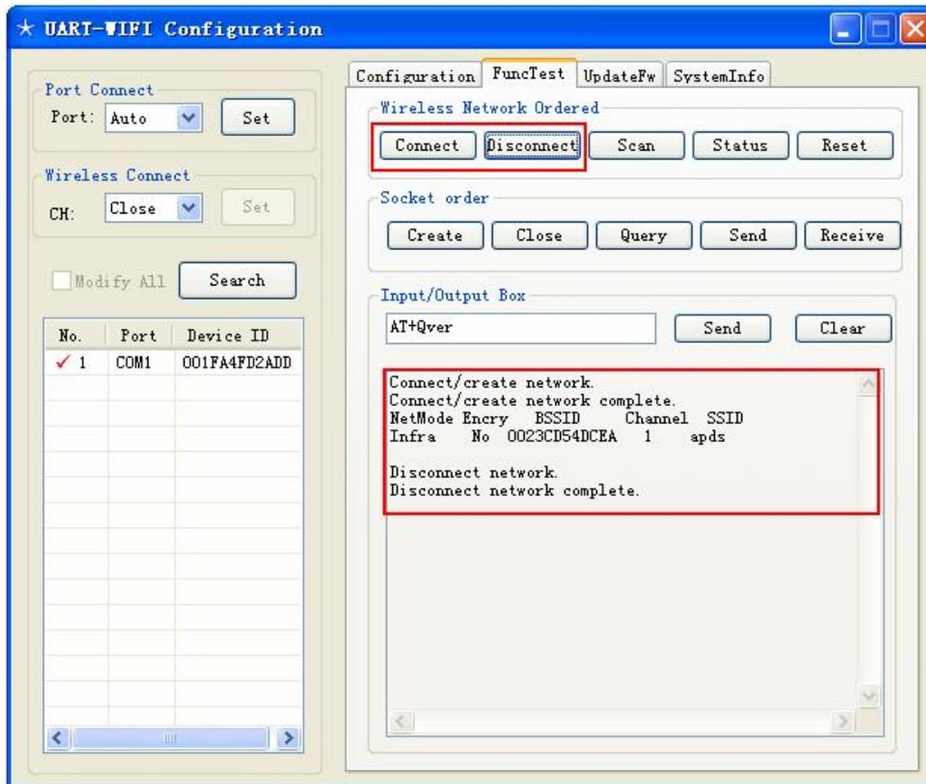
figure5-10 join/disconnect network
