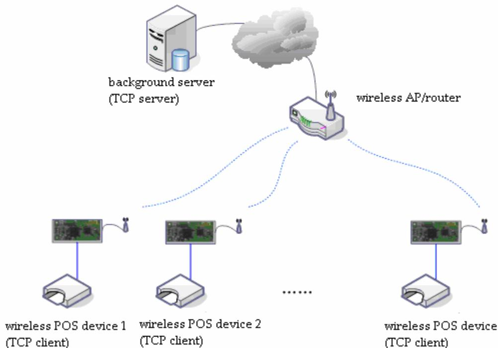
Figure 4-6 The networking of active serial device
