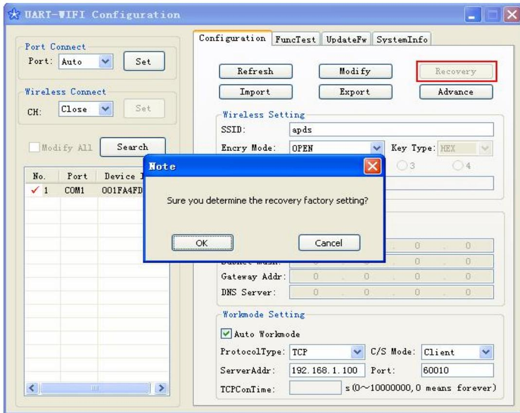
figure5-6 sketch map of restoring to factory setting
